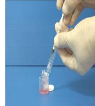
Aspirate the sample into the pre-warmed testing capillary
