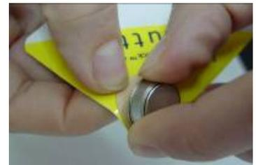
Figure 2: Remove the I-button from its card
