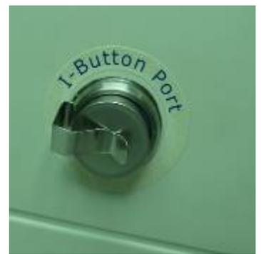
Figure 5: Correct placement of the I-button in the port
