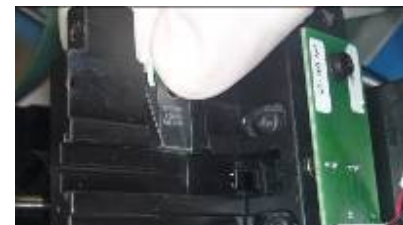
Figure 8: Insert the cover sensor into the optical block
