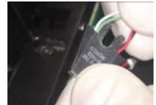
Figure 7: Install the capillary sensor cover
