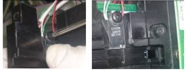
Figure 9: Partially close the screw
