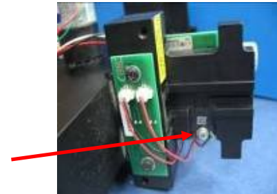
Figure 5: Release the capillary sensor screw
