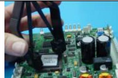
Fig. 4: Remove the damaged processor
