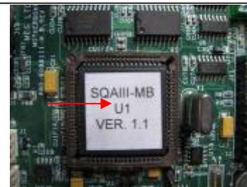
Figure 7: Re-seat the processor
