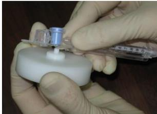
Reposition the blue valve with the jig
