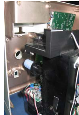
Figure 4: Release the optical assembly
