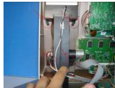
Fig. 3: Unscrew the optical column
