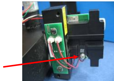
Figure 5: Release the capillary sensor screw
