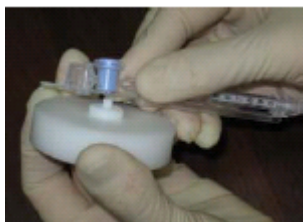
Repositioning the blue valve with the jig
