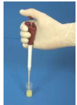
Figure 2: Aspirate the required sample volume
