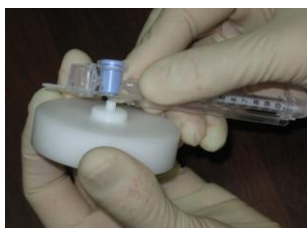
Reposition the blue valve with the jig
