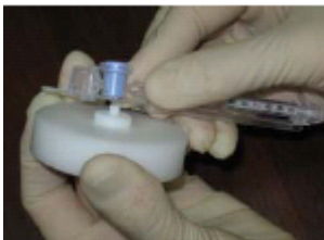
Repositioning the blue valve with the jig
