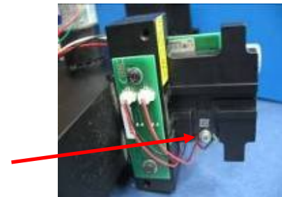
Figure 5: Release the capillary sensor screw
