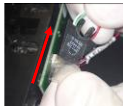
Figure 7: Install the capillary sensor cover
