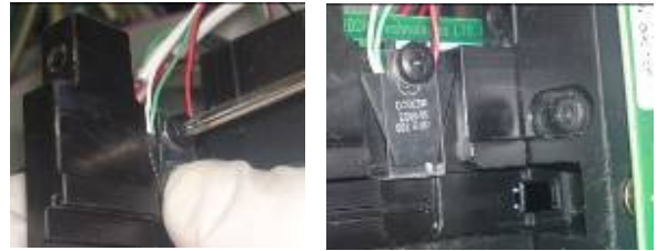
Figure 9: Partially close the screw
