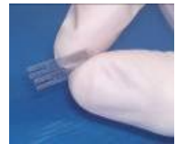
Figure 6: Fold the capillary sensor cover
