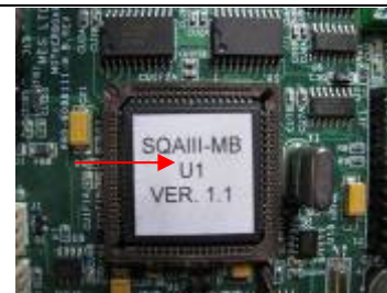
Figure 7: Re-seat the processor
