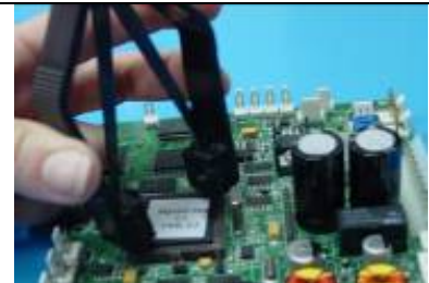
Fig. 4: Remove the damaged processor
