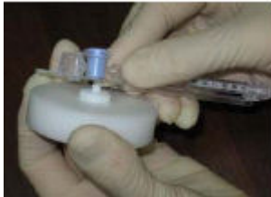
Repositioning the blue valve with the jig
