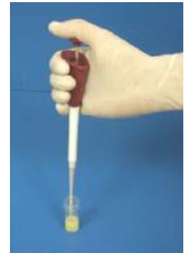
Figure 2: Aspirate the required sample volume
