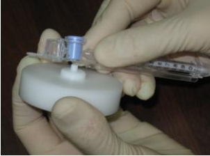
Reposition the blue valve with the jig
