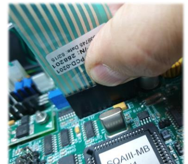
Verify firm connection of keypad cable
