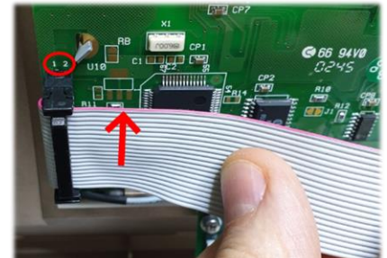
Note the correct alignment of the red line on the flat cable
