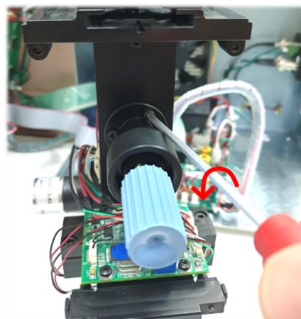
Disconnect the focus knob
