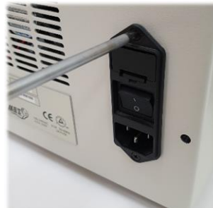
Unscrew the power inlet screws
