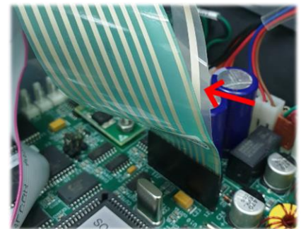
Plug the keypad connector and verify correct orientation
