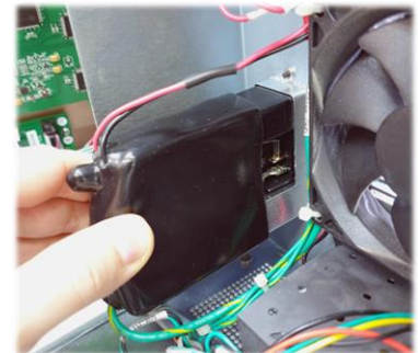
Remove the rubber cover to expose the connectors
