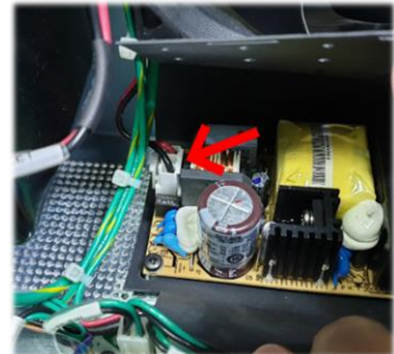
Check the voltage in the input connector
