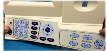
Attach the new keypad
