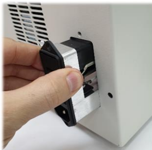
Gently pull the power inlet out the rear panel
