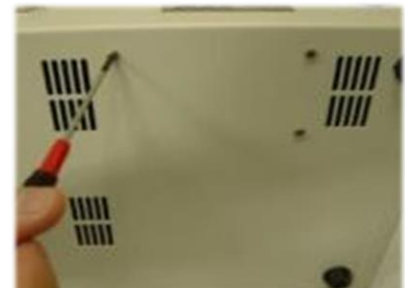
Unscrew the Power Supply Unit (PSU)
