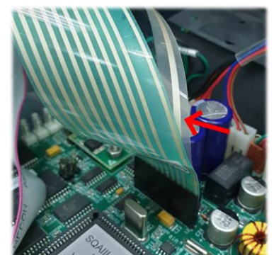
Verify the cable correct orientation
