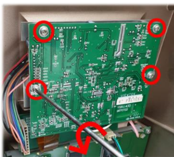
Remove the screws (for SQA-Vs with SN 1504 and below)
