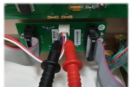
Check voltage on J3 connector
