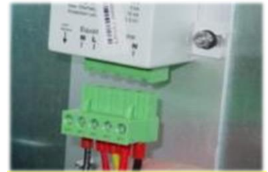
Pull down and unplug the connector
