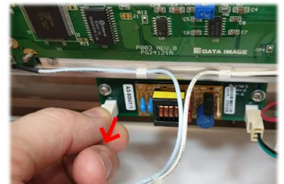
Disconnect the backlight power cable
