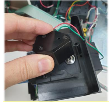
Remove the old Visualization LED housing
