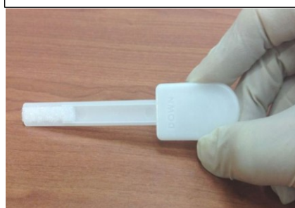
図 5: 挿入—繊維素材面が下側
