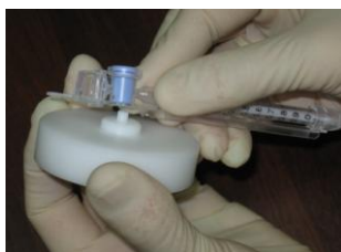
Reposition the blue valve with the jig
