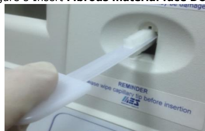
Figure 6 Insertion of drying paddle
