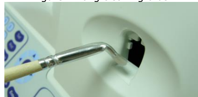
Figure 2 Cleaning lower chamber
