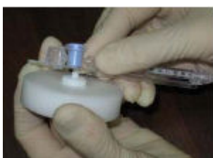
Repositioning the blue valve with the jig
