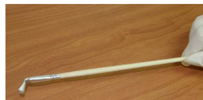
Figure 1 Pinceau long de nettoyage
