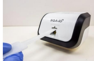
Fig. 5 Insert cleaning paddle down and up
