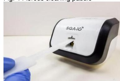
Fig. 5 Insert cleaning paddle down and up
