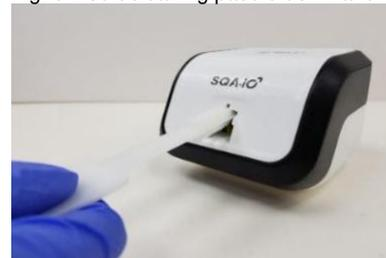
Fig. 6 Dry the testing chamber with sponge
