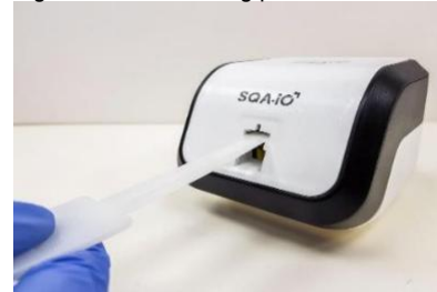
Fig. 5 Insert cleaning paddle down and up
