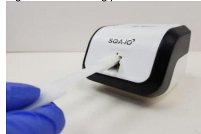
Fig. 6 Dry the testing chamber with sponge
