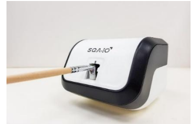
Fig. 2 Clean the chamber
