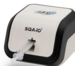
Fig. 5: Insert capillary into SQA-iO
