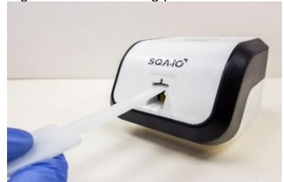
Fig. 5 Insert cleaning paddle down and up
