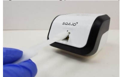
Fig. 6 Dry the testing chamber with sponge
