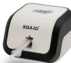
Fig. 5: Insert capillary into SQA-iO
