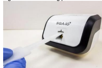
Fig. 5 Insert cleaning paddle down and up
