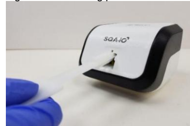
Fig. 6 Dry the testing chamber with sponge
